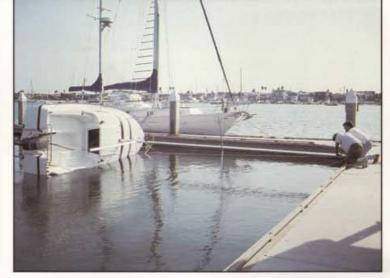
It takes 90 lbs at the top of the mast to hold the boat on its side like this. The 800 pounds of water ballast instantly rights the boat when the mast is released.
