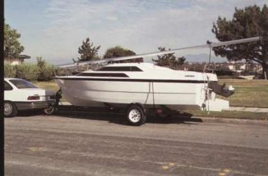
The 19 will fit in a standard garage. The total width is less than 8' and it can be legally towed anywhere. Many states still require expensive and complicated permits for trailering boats over 8' wide.
