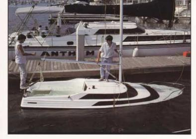
The solid foam flotation will keep it afloat if flooded or damaged. This is what it looks like filled with water. It beats swimming. Other boats would simply disappear.
