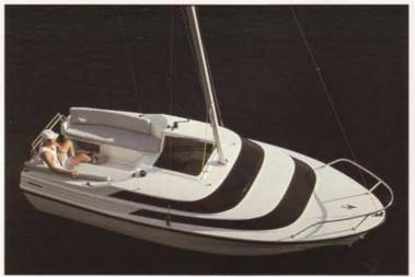
The cockpit is large, comfortable and self bailing. If water comes aboard, it quickly drains out the back without getting inside the boat. This is a safety feature (a swamped boat is no joy) and a convenience (bailing out a week's worth of rainwater is no fun either).
