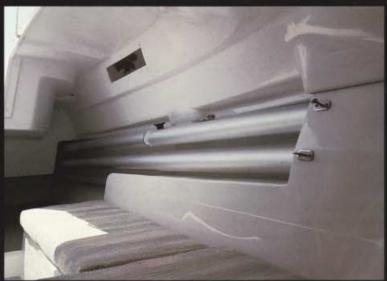
One person can rig the boat, launch it at any convenient ramp and sail away in 10 to 15 minutes. We provide a simple, effective system for raising and lowering the mast. It is easy enough for a kid to do. The mast separates into 2 sections and can be stored in an out-of the way location in the cabin, as shown in the photo on the right. The mast joint is stronger than the mast itself, and assembling the rig is quick and easy.
