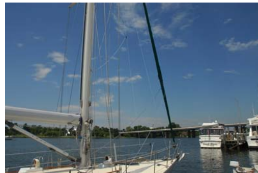
Two dipole antennas visible in this image. Coax leading to 20 meter dipole on port side bow. 8 MHz dipole is visible on starboard bow with the coax feed at the top of the image.
