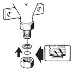
**Installation should be done with the valve upside down.** Place the diaphragm in the cover. Ensure that the entire diapragm is placed in the right location. The diaphragm must not be trapped by the gasket. Insert the gasket and screw on the cover.
