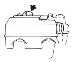
Check the engine oil level. This should be within the area marked on the dipstick. Fill with oil when necessary through the oil filler.
