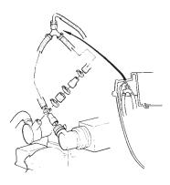
If the engine has a vacuum valve it must be taken apart twice a season or whenever leaks occur.
