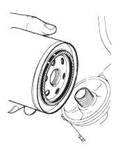
Change the oil filter. The oil filter is to be changed the first time after 20 hours of operation and then after every 200 hours of operation. Screw off the old filter. If the oil filter is difficult to unscrew, there is a special tool which can be used.
