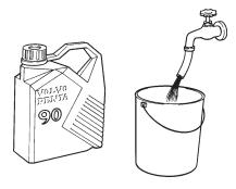
Mix a 50% mixture of fresh water and corrosion-protective anti-freeze.
