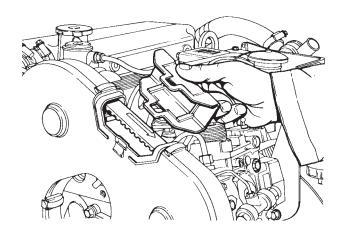
Checking the overhead camshaft drive belt. The toothed drive belt which drives the camshaft should be checked and adjusted by an authorized workshop.
