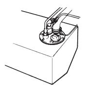
Drain off any water or sediment from fuel tanks. Top up all fuel tanks to prevent condensation during storage period.
