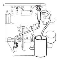
Change the engine oil. The oil is to be changed in new or reconditioned engines after the first 20 hours of operation and then after every 200 hours of operation.
