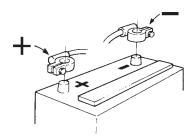
Check that the batteries are fully charged. Smear the terminals with pole grease. Connect the battery cables.
