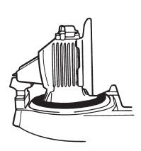
In boats fitted with S-drive, the rubber seal between the drive and the bedding should be checked carefully. **The seal should be changed every seven years.** This should be done by an authorized Volvo Penta dealer.
