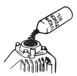
Then reinsert the plug and fill up with oil. Make sure that the oil level is between the maximum and minimum levels indicated on the dipstick. Note: do not exceed the maximum level. See "Technical Data" for type and volume of oil to be used.
