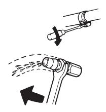
Check the tightening of all hose-clamps. Check that all drain-cocks are closed and tight. Clean the engine and reverse gear on the outside. Check the exhaust-hoses. Install the impeller.
