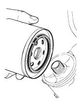
Change the oil filter.\* If the engine is fitted with an S-drive this should be drained when the boat is laid up. Fill up the engine and reverse gear to the correct level with Volvo Penta diesel engine oil\*, which also has corrosion protective properties. Start the engine and check for leaks. The engine is now ready to run on this oil next season.
