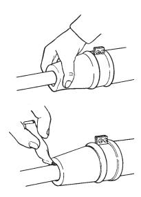
If the boat is equipped with a propeller shaft seal of rubber, the following procedure should be observed after launching:
