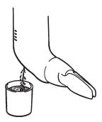
Change the oil in the S-drive. Remove the dipstick. Remove the plug under the propeller gear housing and allow the oil to run out.
