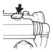
Fill-up the freshwater system to the correct level. Fill-up through the filler-hole on top of the heat exchanger with a 50% mixture of freshwater and rust-proofing ethylene glycol or additive.
