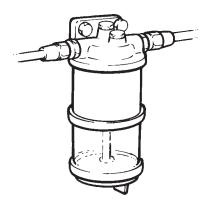
Change the insert in any extra fuel filter fitted.
