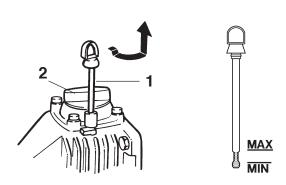
Check the oil level in the reverse gear or S-drive
