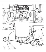
Drain water from the fuel filter. Open the venting screw (1) approx. 3 turns. Then open the drain screw (2) and drain the fuel/water into a suitable container. Tighten the drain screw and vent the fuel system. See "Venting the fuel system".
