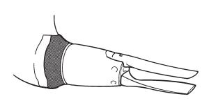
Check the zinc ring\* on the S-drive and replace if it is consumed more than 50%. Otherwise clean the anode (also a new one) with an emery cloth to remove the oxide layer. NB. This should be done shortly before launching.
