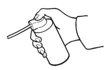
Clean the outside of engine, and reverse gear/S-drive. Touch-up any bare patches in the paintwork with Volvo Penta original paint. Spray the components of the electrical system, and all the control components with anti-moisture spray. All engine control linkages should be inspected for wear, properly adjusted and protected from corrosion.
