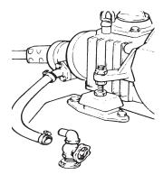
Loosen the hose between the sea-water intake and the reverse gear/S-drive. Connect a hose and put the other end in a bucket with fresh water. Provide for the topping-up of fresh water into the bucket. Run the engine at fast idle a few minutes.
