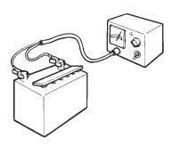
Remove the batteries from the boat. Clean them and store them in a cool, dry place. Check that the batteries are well charged. Trickle charge them according to the manufacturer's instructions (a flat battery can easily be damaged as a result of freezing).
