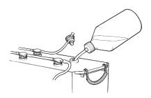
Check the level of electrolyte in the battery (batteries). The level should be 5–10 mm (3/16"–3/8") above the cell plates in the battery. If necessary, topup with distilled water.
