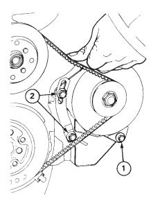
Repace the v-belt. Loosen the alternator mounting bolts 1 and 2 and slip off the belt. Clean the belt groove on the pulley before fitting the new belt. Tension the belt in such a way that it can be depressed 10 mm
