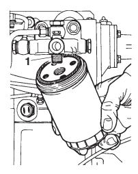
Change the fuel filter. Unscrew the fuel filter using a filter remover or other suitable tool. Ensure that the nipple (1) is firmly seated in the filter head. Screw on the new filter and tighten by hand. Vent the system, start the engine and check for any leakage
