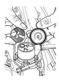
Clean the feed pump filter. Remove the cover and remove the filter.
