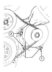
Check/tension the drive belt. Tension the belt in such a way that it can be depressed 10 mm (3/8") between the pulleys. Change the belt if it looks worn or is cracked. Loosen the alternator mounting bolts 1 and 2 when tensioning or changing the belt.
