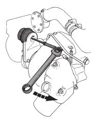
Check the turbochargers wast gate valve (TMD22) by turning the shaft according to the picture.
