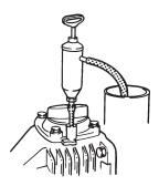
Check the oil-level and check also for leakage around the filter.
