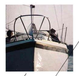
**Bow Pulpit** – A welded stainless steel pulpit gives extra support when working with the jib, anchor, or docklines. Lifelines are standard on the O'Day 23 and 25.
