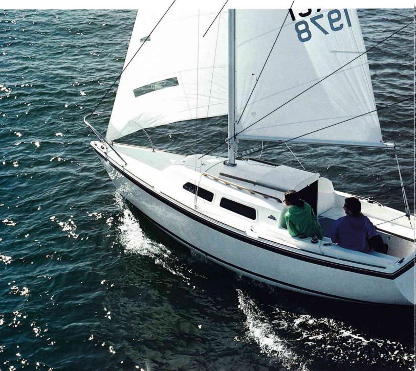
Forward Hatch – Mounting the hatch flush means easier tacking with fewer hang-ups for the jib, longer life for sails and a comfortable place to sit up forward. It also means less chance for leaks.
