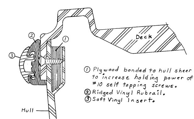
The hull/deck joint is bedded and bonded together with a polyurathane adhesive. The deck is mechanically fastened with #10 Stainless Steel screws on 6 in. centers.
