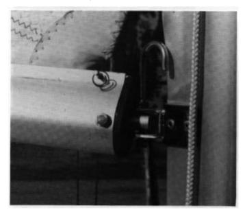
Photo 23 Connect boom to mast
