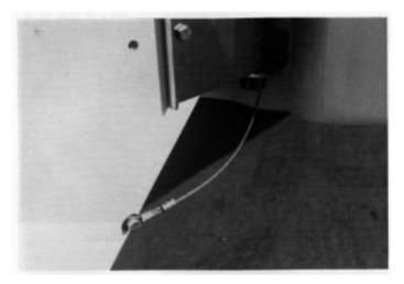
Photo 35, Rudder hold down wire attachment
