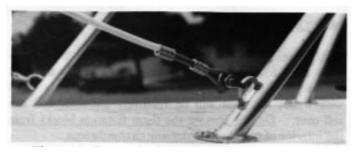
Photo 41 Forward safety rail connection
