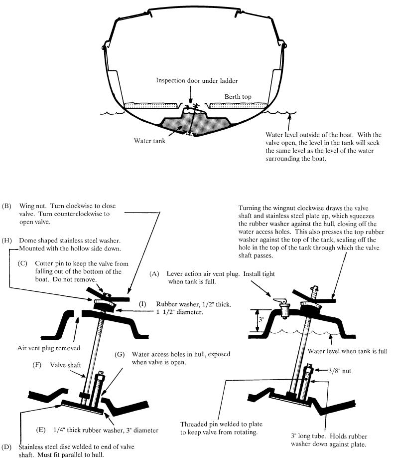
necessary to use tools. As you tighten the wingnut, the valve shaft (F), plate (D) and seal (E) are pulled up tight against the hull, sealing off the water access holes (G) and trapping the water in the ballast tank. As the wing nut is tightened, the cone shaped washer (H) and rubber seal (I) are pressed tight against the top of the water tank, sealing the top.
