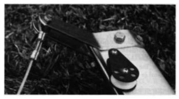
Photo 2 Rear mast support wire attachment (backstay)
