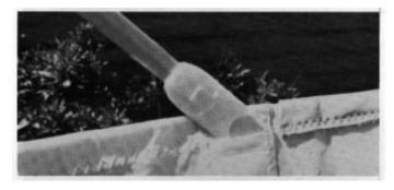
Photo 29 Batten, partially inserted
