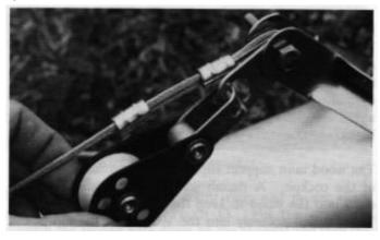
Photo 4 Forward mast support wire and jib pulley
