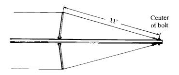
Drawing 8 Spreader tube ends: wire position
