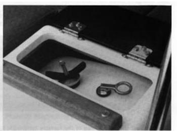
Photo 22. Water Valve and air vent.
