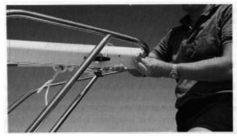
Photo 11 Mast bolted to front rail
