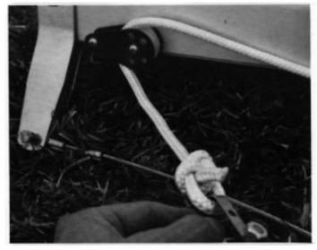
Photo 9 Mainsail hoisting rope
