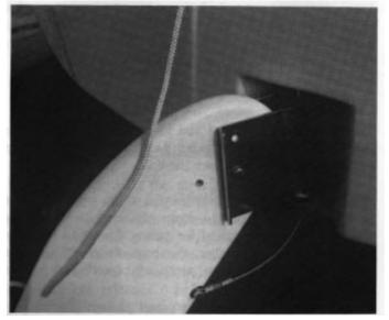
Photo 34 Rudder attachment
