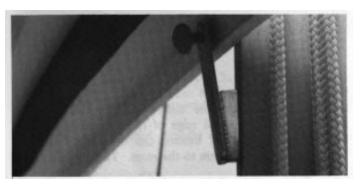
Photo 37 Securing the pop top in the up position
