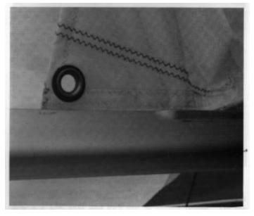
Photo 25 Attaching the mainsail to the boom
