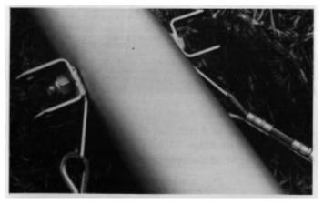
Photo 5 Middle side support wires (lower shrouds)
