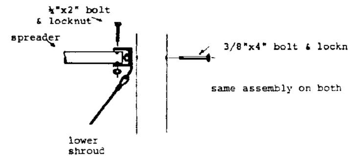
Install the lower shrouds and spreaders. Connect the spreaders to the upper shrouds. Make sure the spreader and fittings are clamped securely to the upper shrouds. On the 21 and 22 the backstay bent tang slips over the 3/8" bolt protruding from the rear of the masthead and is held firmly in place with a 3/8" locknut. On the 25, the backstay wire loop bolts (with a 1/4" x 1 1/2" bolt and locknut) between the rear holes in the masthead fitting. Make sure the nut is fully engaged in the threads.
