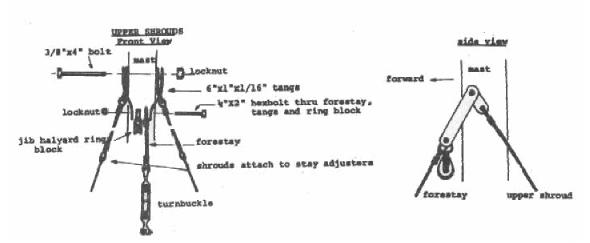
Make sure the tangs are mounted with the smooth center surface of the tang contacting the mast. If the tangs are mounted wrong side out, the edges of the tangs may cut into the mast. Tighten the bolts snug, but not tight enough to deform the mast and fittings.
