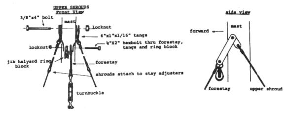
Make sure the tangs are mounted with the smooth center surface of the tang contacting the mast. If the tangs are mounted wrong side out, the edges of the tangs may cut into the mast. Tighten the bolts snug, but not tight enough to deform the mast or fittings.
