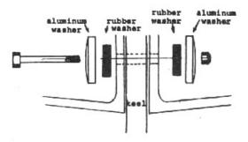
When the keel pivot bolt is re-installed, make sure that it passes through the hole in the keel.
