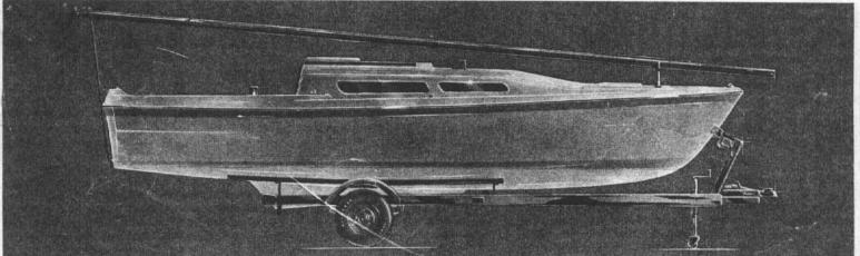
Length 24'11" Beam 7'11" Weight 2100 lbs. Draft— Keel Down 5'8" Draft-Keel Up 1'10" Keel Weight 625 lbs.
