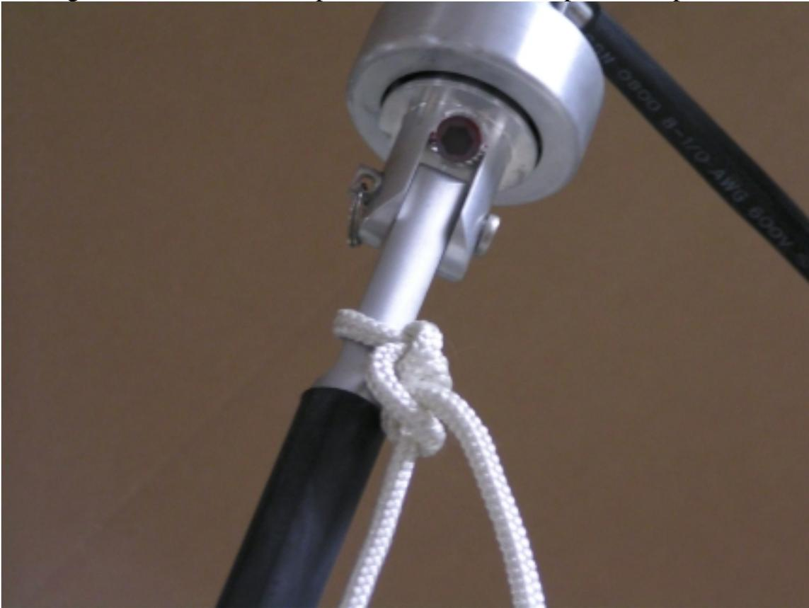
3. With a short piece of 1/4” dia. double braid line, attach the tack of the spinnaker to the holes in the spinnaker swivel. (see picture). The length of line used will help determine the sail shape of the spinnaker.
