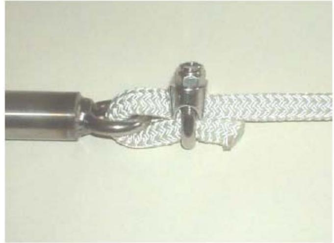
6. Attaching the tow rope to the turbine
