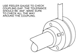
NOTE: CHECK COUPLING GAP WITHOUT COUPLING BOLTS IN PLACE.
