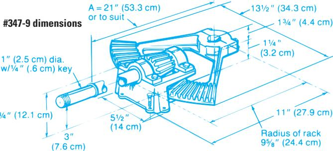
NOTE: The "A" dimension is the distance between the centerline of the rudderpost to the aft side of the wheel.
