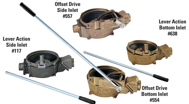
Manual 30 GPM Diaphragm Pumps are available in four models with either side inlet or bottom inlet chambers and lever action or offset drive sockets. The choice of model is based on where you want to locate the pump on the boat. The Offset models facilitate mounting the pump behind a bulkhead. A 32" plated steel handle comes with every pump. It is used for easy stand up pumping. A stainless steel handle is optional.
