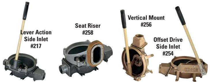
18GPM Manual Diaphragm Pumps are offered in varying configurations to facilitate installation based on where you want to locate the pump on the boat. The #254 Offset Pump facilitates mounting the pump behind a bulkhead, the #256 Vertical Mount Pump allows mounting the pump on a wall and the #258AL is ideal for mounting behind a set riser in the cockpit. An 18" aluminum handle comes with every pump. A 32"/81cm handle, available in plated or stainless steel is optional.
