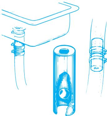
Edson's Anti-Surge Valve controls the flow of drain and bilge water in your boat with a simple floating ball. Use the anti-surge valve wherever the possibility of water backing up in drain lines exists. Ideal for head sinks, galley sinks, and anchor wells that fill when your boat heels over. These valves can also be used in limber holes and grid pan drains to keep bilge water from traveling. Comes complete with two Stainless hose clamps and is available in four sizes.
