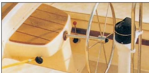
The Island Packet above shows a typical installation of the Edson #317 Compass Pedestal.
