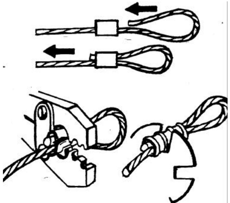
**LAP SPLICE:** After threading the two lengths of cable into the Oval Sleeve, crimping instructions are basically the same as loops. Note, a minimum of two sleeves are recommended and proper tests should be made to determine actual strength of the splice. Leave the usual 1/8" of cable protruding from the sleeve and allow a space of at least two cable diameters between the sleeves. Gauge as usual.
