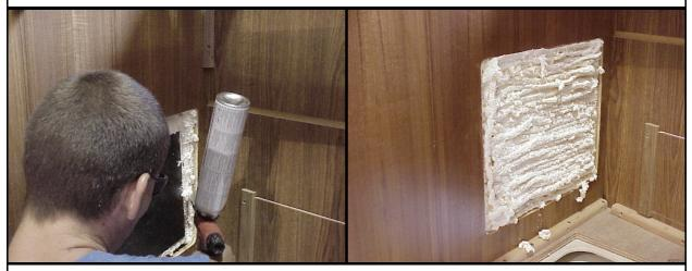
After the icebox face and the forward galley bulkhead have been installed have the insert cover ready to install. Fill all voids around the insert flush to the wood face minimum to approximately 1/4" proud then apply a layer of foam on the back of the insert so it completely covers the back.
