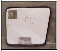
Glue the rubber gasket around the perimeter of the icebox lids with 401 loctite so the open side of the gasket faces in and the seam is on the hinge side of the lid. Glue the seam together with 401 loctite.
