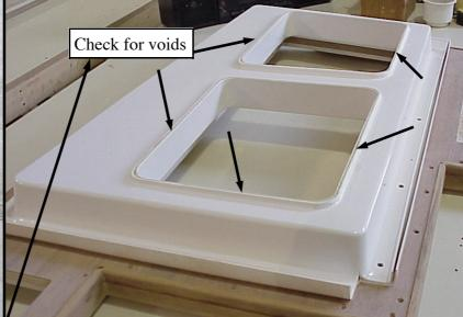
After checking for voids lay center the openings in the icebox top insulator with the holes in the galley top then mark the perimeter of the icebox top insulator onto the bottom of the galley with a pencil.
