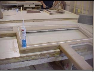
Caulk (using 5200) generously just inside the pencil line that was marked earlier on the bottom of the galley top.
