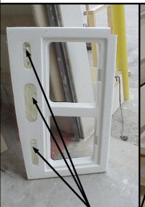
After the access holes of the icebox top insulator have been cut off check to make sure the part is completely filled with foam and there are no voids around the cut edge. If voids are found reject the part.
