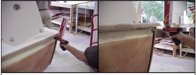
On the back side of the icebox place the foam gun nozzle all the way in the void between the top of the icebox and the side of the galley and inject foam while pulling the foam gun out, filling the void. Do this procedure on both sides. CAUTION: Do not over fill as foam will expand and distort the outer bulkheads.
