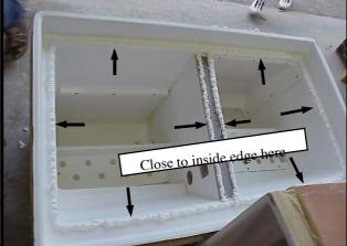
Caulk (733 white caulk) generously along the inside edge of the second tier from the top and both edges on the top of the divider.
