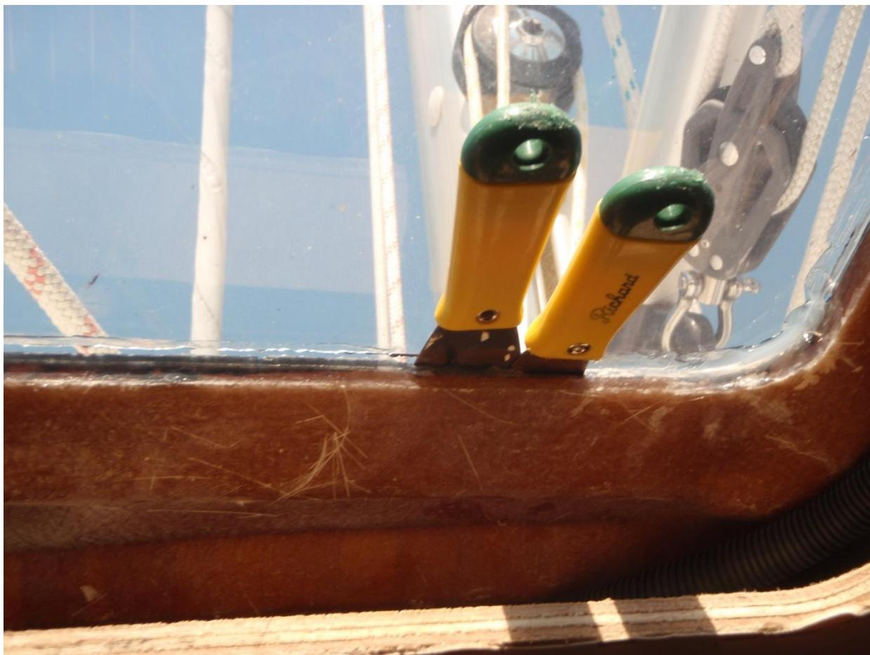
As the sealant started to release, the window gently moved upwards. Went back to the cockpit and gave the winch 2 clicks only, just to take up the tension. Went back below, and removed more sealant, and the window kept lifting.
