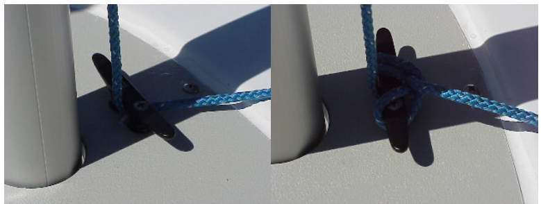
After the sail is raised, run halyard forward through cleat and tie off .
