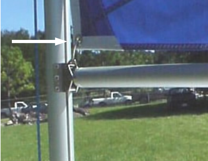
Attach mainsail tack to hook on gooseneck.
