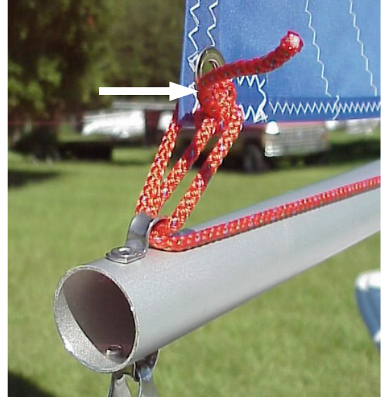
Attach outhaul to mainsail clew. Lead through outhaul bale. Pull to tighten and secure on outhaul cleat.
