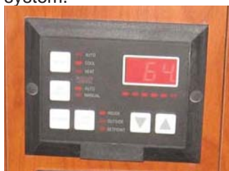
Fig. 8.4 shows one of three air conditioning unit wired remote control panels. for more detail information, please refer to the A/C owner's manual
