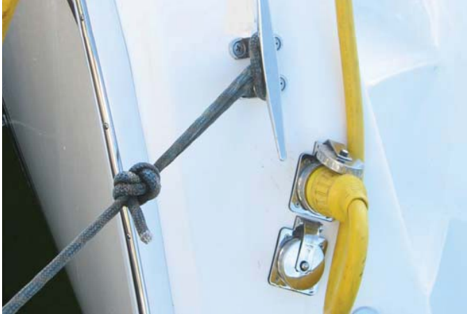
Fig. 8.1 Shown is the aft shore power connection.
