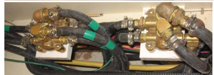
Fig. 5.6 Fuel tank selection control valve
