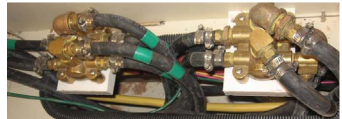
Fig. 5.6 Fuel tank selection control valve
