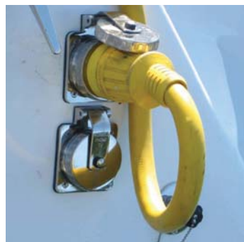
Fig. 8.5 the stainless shore power connector located on transom port side next to mooring cleat. the upper connector is for AC connection, and the lower connector is for TV antenna connection.
