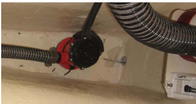
Fig.10.6 shows the main bilge pump locates in main bilge compartment
