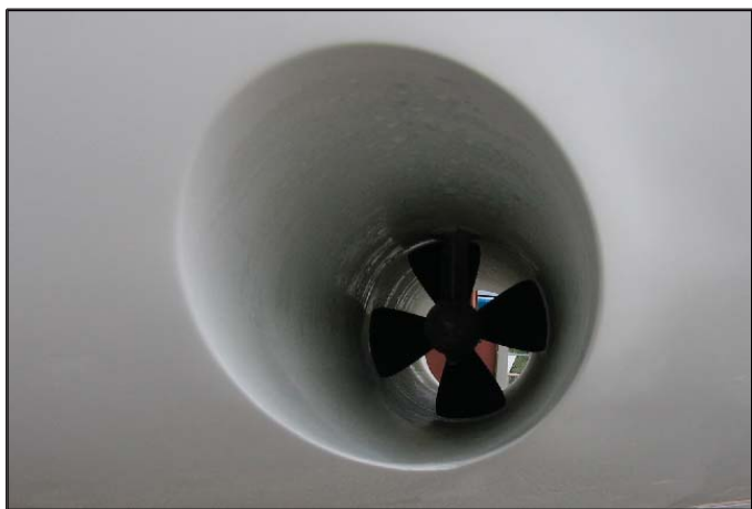
Fig. 6.12 bow thruster tunnel
