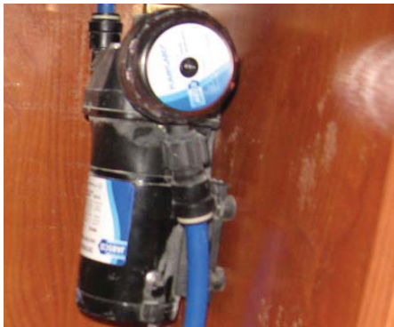
Fig. 9.3. Replace the strainer periodically for better performance of the entire fresh water system. The water pump unit with strainer locates underneath the galley shelf.
