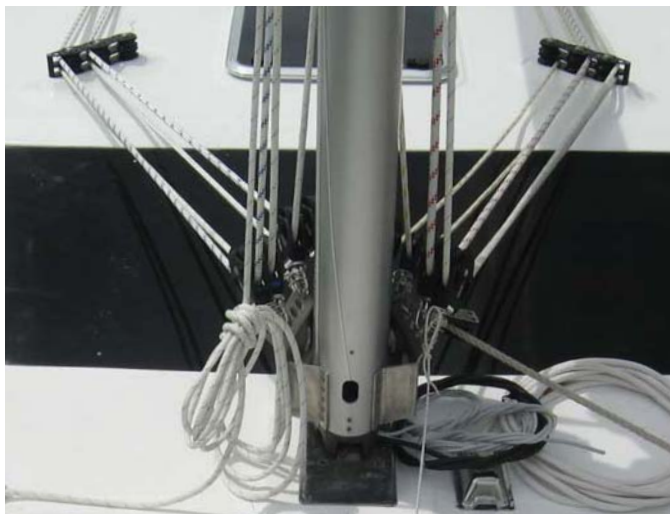
Fig. 12.1 shows the front view of mast with running rigging installed on the 50c.c
