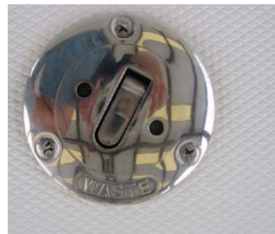
Fig. 10.12 shows waste holding tank pump out fitting. Only pump out sanitation material at pump out station where is available
