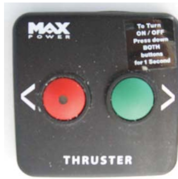
Fig. 6.13 The bow thruster control panel located on cockpit pedestal. See instructions on Bow Thruster user's manual for bow thruster operation. Refer to Bow thruster owner's manual for more details
