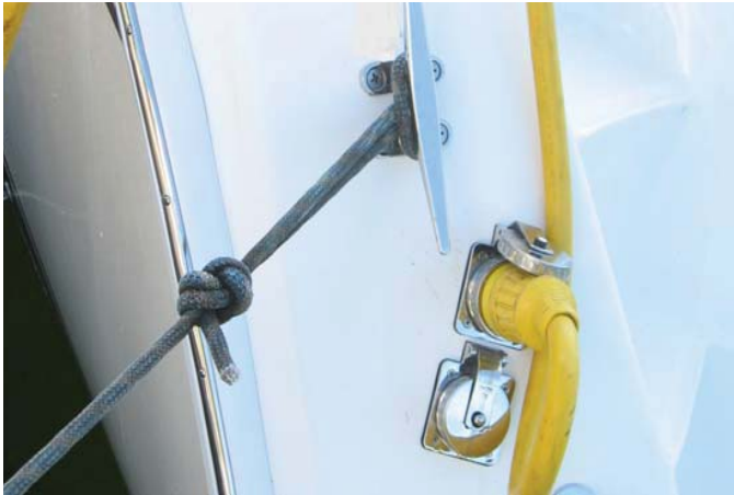
Fig. 8.1 Shown is the aft shore power connection.
