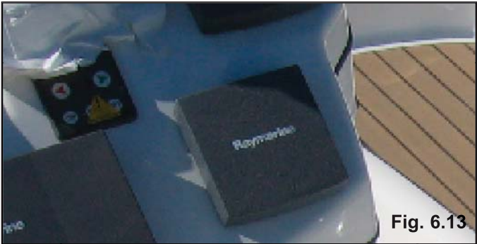
Bow Thruster Controls Located at the helm Left button moves the bow port, the right button moves the bow starboard.
