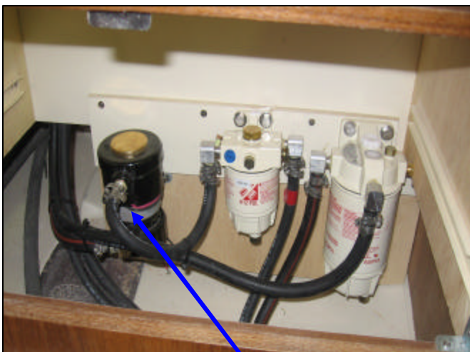
Inside QB Bunk port lower drawer shelf , engine fuel filter, genset fuel filter and fuel pump
