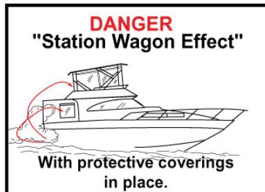
Figure 4.6. When protective weather coverings are in place, engine or generator exhaust from your boat, while docked and/or running, can cause excessive accumulation of Carbon Monoxide gas within the cabin and cockpit areas of your boat. Always provide adequate ventilation when the weather coverings are in place and either the engine or generator are running.
