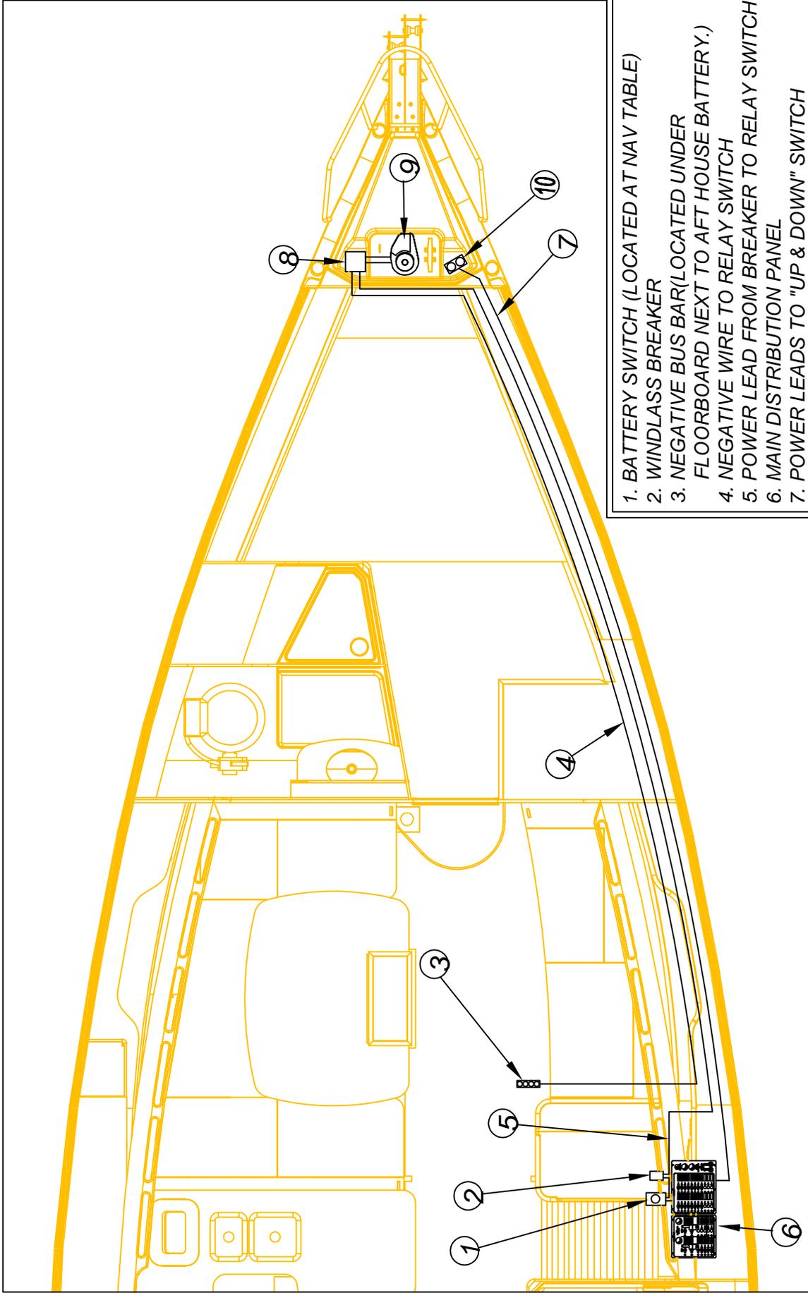
1. BATTERY SWITCH (LOCATED AT NAV TABLE)
