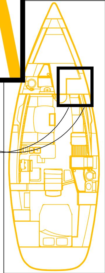
**NOTES: WHEN AN ICE MAKER IS OPTIONED, A 15 amp BREAKER IS INSTALLED @ THE MAIN BREAKER PANEL, LOCATED @ NAV STATION.**
