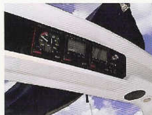
Integrated Mainsheet arch / instrument panel with lights, stereo speakers, dodger & bimini support.
