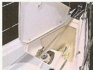
Anchor well w / dual anchor rollers, separate rode storage and optional windlass.
