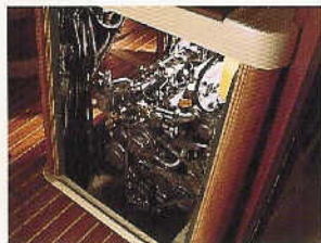
50hp freshwater cooled diesel w / 50 gal. fuel tank.
