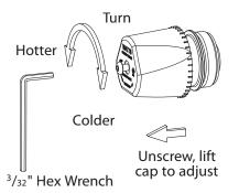
Figure 9.5.0 - Temperature Adjustment
