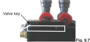
Shows the valve key horizontal to the line, or closed.
