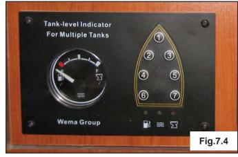
The power switch turns the monitor on, then select the tank you want to monitor. The gauge on the left will show the amount remaining in the tank.
