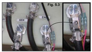
In Fig.5.3 you can see the fuel supply fittings. The photo inset shows the close-up of the fuel valve. See Fig.5.5 for the function of the fuel valves.
