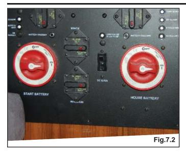
The battery switch panel houses the breakers for some of the main components in your DC system. The breaker controls are marked at the switch panel, and control systems or components on your boat that require a connection that remains energized even through the Main Panel may be de-energized.
