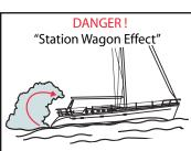
**Figure 4.5.** Engine or generator exhaust from your boat while underway and operating with a high bow angle can cause excessive accumulation of Carbon Monoxide gas within the cabin and cockpit areas of your boat. Always provide adequate ventilation and redistribute the load to lower the boat angle.
