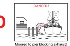
**Figure 4.3**. Blocked hull exhaust outlets near a pier, dock, seawall, bulkhead or any other structure can cause excessive accumulation of Carbon Monoxide gas with the cabin areas of your boat. Be certain hull exhaust outlets are not blocked in any way.
