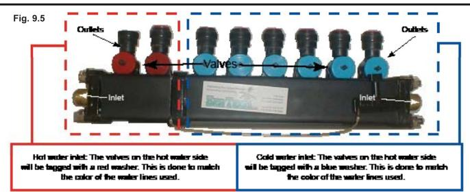
Note: Actual water manifolds may vary in detail from the one pictured above. The manifold is based upon the amount of components, or systems being fed from the manifold.
