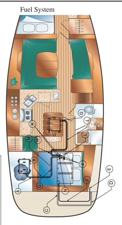
ENGINE FUEL RETURN LINE 5/16" (.79cm) ENGINE FUEL SUPPLY LINE 5/16" (.79cm) ENGINE AND GENERATOR FUEL RETURN PORTS FUEL CUTOFF VALVES A GENERATOR RETURN FUEL LINE 1/4" (.66cm) B GENERATOR FUEL SUPPLY LINE 1/4" (.66cm) C FUEL FILL HOSE 1-1/2" (3.8cm) D FUEL FILL (ON DECK) E FUEL VENT (ON DECK) F TUEL VENT HOSE 5/8" (1.6cm) L FUEL LEVEL SENSOR M GENERATOR FUEL PUMP N OPTIONAL HEATER FUEL SUPPLY LINE FUEL FILTER/WATER SEPARATOR
