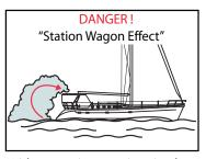
**Figure 4.6.** When protective weather coverings are in place, engine or generator exhaust from your boat, while docked and/or running, can cause excessive accumulation of Carbon Monoxide gas within the cabin and cockpit areas of your boat. Always provide adequate ventilation when the weather coverings are in place and either the engine or generator are running.
