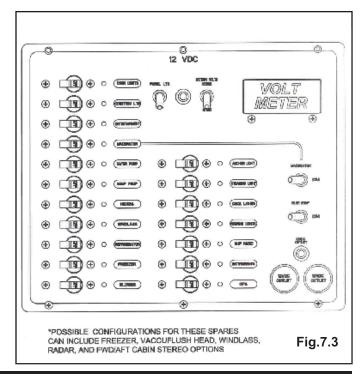
You can view the parts of the DC side of the main control panel here (Fig. 7.3). Notice the battery selector switch at the top left, when switched on the respective voltage of the battery is shown on the right by the digital volt meter. Indicator lights are built into most switches and alert you that the selected system is powered.
