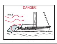
**Figure 4.7.** While underway or drifting slow speed can cause co buildup, add a tailwind and this can intensify the effect.
