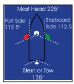
The arc of the lights and color allows you to determine the direction a vessel is moving. How good are your lights? You should test them to see how visible you might be at night. Whether on a trailer or at the marina, switch on your lights and see how well they can be seen. Walk away from the boat or row away, if you are at anchor or at a mooring, and see how visible the lights are as you move further away. How easy are they to see against the background of lights on shore?
