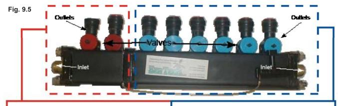
Hall water inlet. The valves on the hot water side. will be tagged with a red washer. This is done to match the color of the water lines used.
