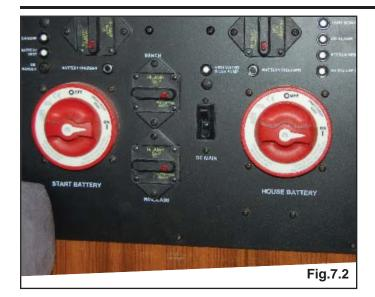
The battery switch panel houses the breakers for some of the main components in your DC system. The breaker controls are marked at the switch panel, and control systems or components on your boat that require a connection that remains energized even through the Main Panel may be de-energized.
