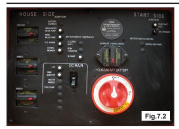
The battery switch panel houses the breakers for some of the main components in your DC system. The breaker controls are marked at the switch panel, and control systems or components on your boat that require a connection that remains energized even through the Main Panel may be de-energized.
