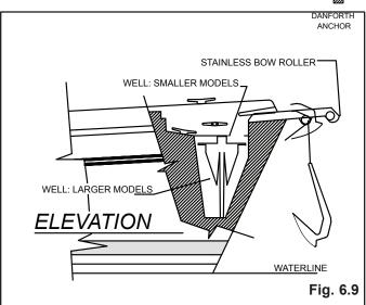
Fig 6.9 shows you a profile view of the anchoring, and windlass system. This illustration shows the smaller and the larger anchor well, in relation to the location.
