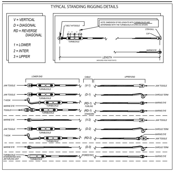
Figure 12.12 Standing Rigging Details
