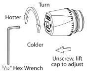
Figure 9.5.0 - Temperature Adjustment
