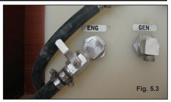
In Fig.5.3 you can see the fuel supply fittings. The photo inset shows the close-up of the fuel valve. See Fig.5.5 for the function of the fuel valves.
