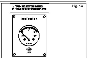
The power switch turns the monitor on, then select the tank you want to monitor. The gauge will show the amount remaining in the tank(s).
