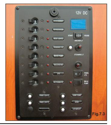
You can view the parts of the DC side of the main control panel here (Fig. 7.3). Notice the battery selector switch at the top right, when switched on the respective voltage of the battery is shown above on the digital volt meter. Indicator lights are built into most switches and alert you that the selected system is powered.
