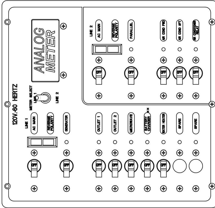
\*\*IF THE BOAT IS EQUIPPED WITH AN INVERTER INSTEAD OF BATTERY CHARGER, THIS BREAKER BECOMES A SPARE.
