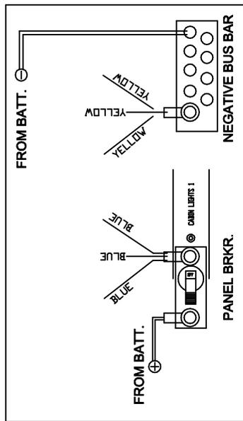
EACH CIRCUIT IN PARALLEL, BLUE (LOAD TO BREAKER) AND YELLOW NEGATIVE TO NEGATIVE BUS BAR (SEE EX.)
