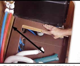
The backside of the shelf fits into a 1/4" dado in the galley so the shelf will need to be pulled towards you before lifting it up out of the way
