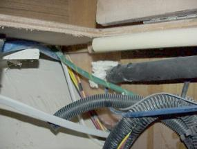
Check the forward side of the hole (it can be seen by opening the bunk lid just forward of the galley) to make sure it has filled completely. After the hole is filled with foam reseal the side of the hole in the icebox with the putty that was removed earlier.
