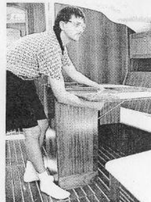
3 WHILE HOLDING HANDLE IN STORAGE BOX LID, RELEASE BOLT LOCATED UNDER THE AFT END OF THE TABLE
