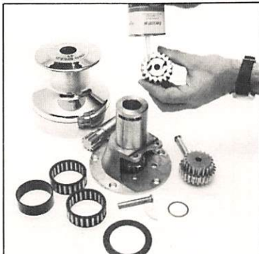
Remove pawl gears and clean. Lightly oil pawls and grease gears.
