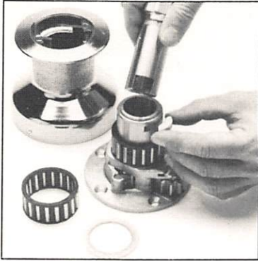
Remove centre spindle key and slide out spindle.
