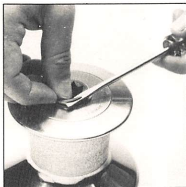
Remove the top circlip with a small screwdriver or knife blade.
