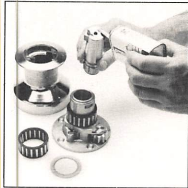
Clean spindle, grease lightly and oil pawls.
