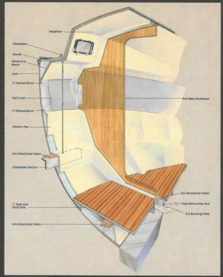
gineered to minimize leaks and act as a spray rail. A custom pre-bent toe rail extrusion is thru bolted providing additional strength and protection. The stanchions are mounted outboard which allows for easier and safer movement about the side decks.
