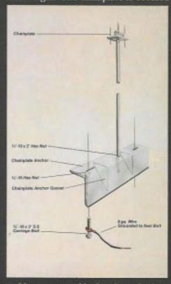
to this system and is then brought thru the deck in one clean penetration, creating more interior space and minimizing deck clutter. The load is then distributed to the hull thru the internal frame and stringer system.
