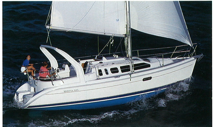
Beam reach or hard on the wind, the 310 has the versatility in the sailplan to do it all. The absence of the backstay allows for a large roach main and a small furling jib. Adjustments are quick and easy.
