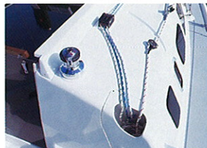
Coaming wells keep the halyards and sheets neat and organized. All lines lead aft to the cockpit to make short-handed sailing easier.
