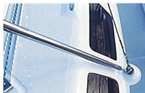
Attachment of the mast struts are secure and inboard to keep the sidedecks free and clear.
