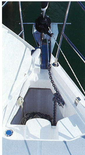
The deep anchor well can hold plenty of rode and chain and provides a mount point for the optional windlass as well as the standard anchor roller.
