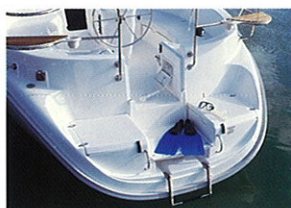
Swimming, diving, or just loading the tender is easy from the walkthrough transom and swim platform.
