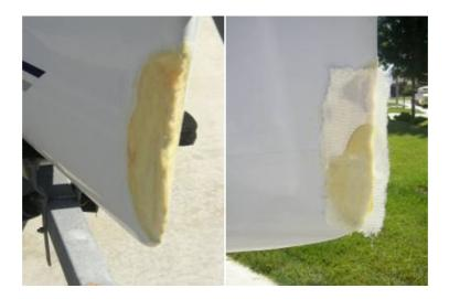
Two part Plexus epoxy is used to firm up the damage and give a smother repair area. Unidirectional cloth is layered over repair area, working the epoxy in well.
