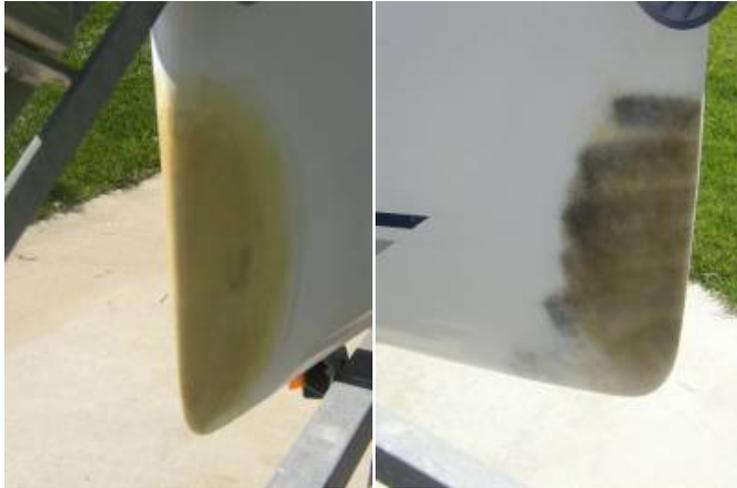
A finish coat of plexus id applied and a light guide coat is used to make sure repair is smooth and sand scratches are removed
