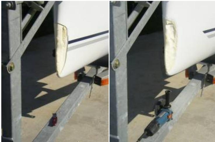
Using a utility knife, cut back to solid. Sand away the loose foam and taper plastic.
