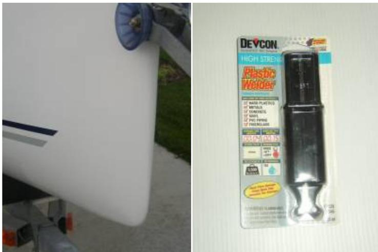
Repair is painted and polished the next day. This is the only place I vary from factory recommendations, I use a two part urethane made by BASF, matched at the local automotive paint store. Plexus is sold under the name Devcon Plastic Welder.
