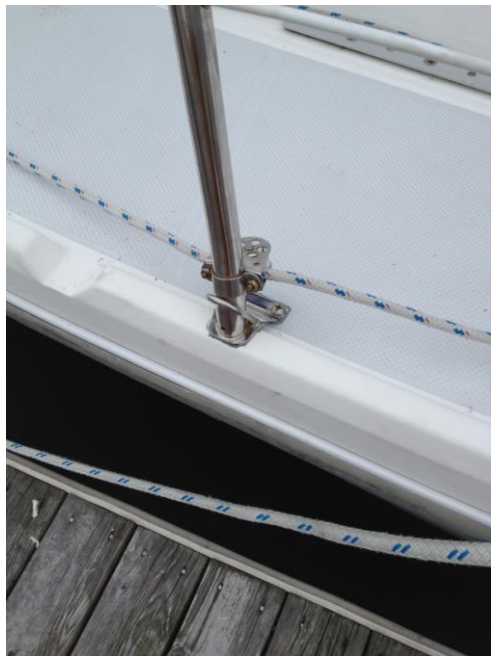
Trim excess butyl tape to make it look nice.
