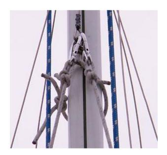
The upper end of the bridle is attached to the main halyard. A short length of line is tied around the mast and through the two carabiners. This line keeps the upper end of the bridle close to the mast.
