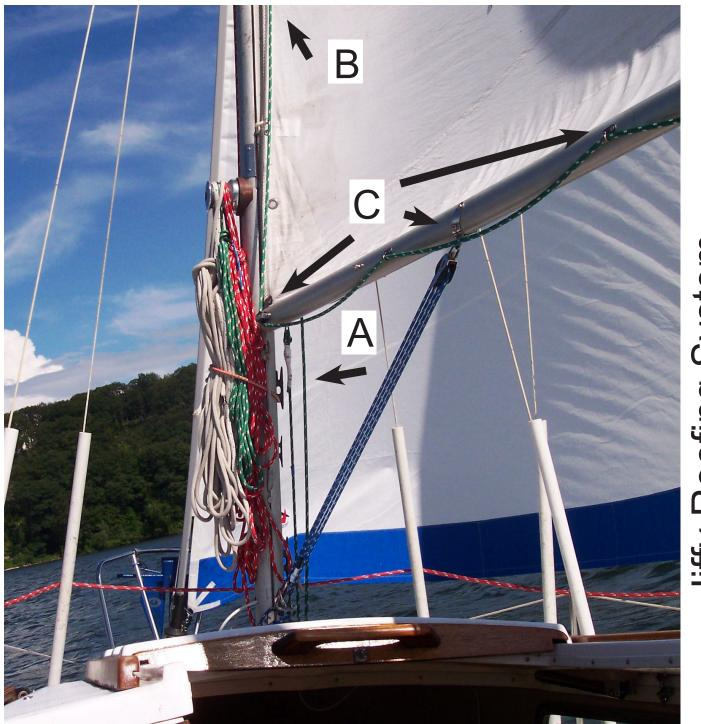
A – Jiffy Reef, comes from starboard rope cleat, through deck organizer, mast base block to reef point.
