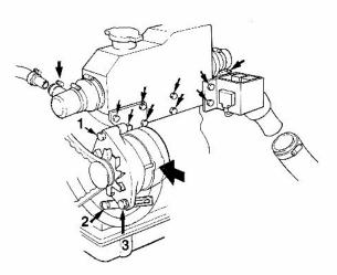
The screws which hold the alternator bracket and electrical distribution box in place also hold the expansion tank/heat exchanger/exhaust pipe (1). Be careful when you take the screws out, the entire package is now loose and is quite heavy. Do not allow it to fall unchecked since the alternator could be damaged.
