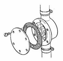
Always use a new gasket between the pump housing and the lid. Install the lid.
