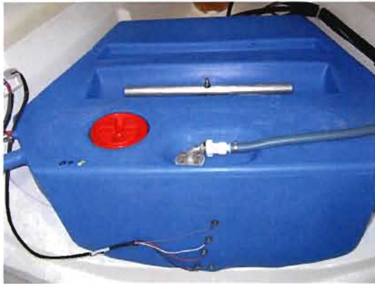
Forward water tank Lay out of: Forward cabin Capacity: 160 liter
