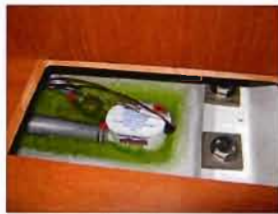
Electric bilge pump Lay out of: Sump Capacity: 70 liter / minute
