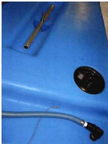
Aft water tank Lay out of: Starboard aft cabin Capacity: 200 liter
